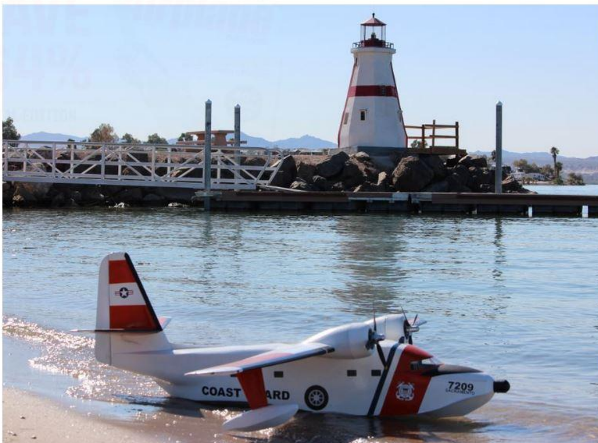
(Above) Monty Welch's Park Scale Albatros in Coast Guard colors. The model is 96" span and is only 10.5 lbs! Electric powered and was built by his wife Lina Welch, truly a family project.
