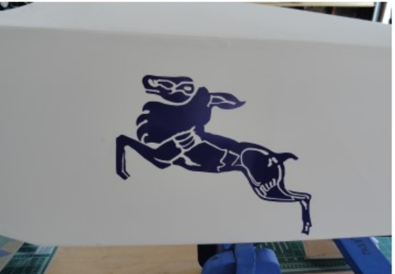
Here I used my vinyl graphic cutter to design this Elk and place the mask on the fuselage. The purple is the vinyl.
