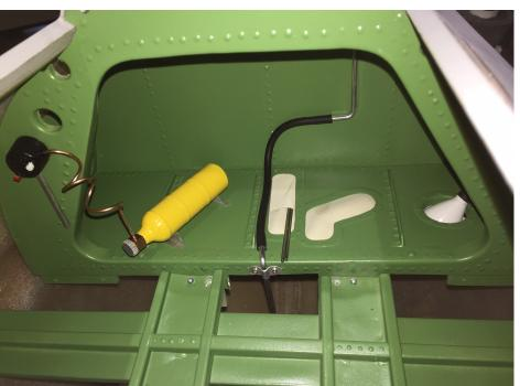
Typical of the cockpit sub-assemblies... parts are individually bagged with an instruction sheet in each bag. The kit to the right builds into the rudder pedals (below). The parts now need to be individually painted before final assembly.
