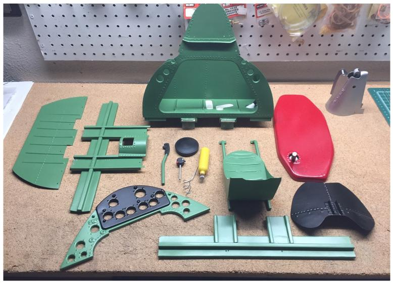
Just some of the cockpit parts, trimmed and painted. Most parts are ABS, but some are cast resin. The resin parts can be hollowed out to reduce weight. Pilot seat and mounting rails (left below). Some added "gingerbread" below...
