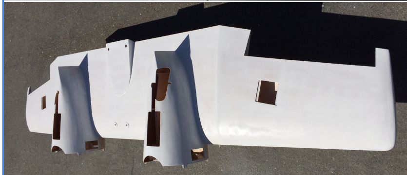
TOP: Top of wing, glassed and sanded. ABOVE: Bottom of wing, freshly primed. RIGHT: Auto spot (glazing) putty applied to every visible low spot, divot, and void. After another sanding and priming, MORE "issues" will be visible!
