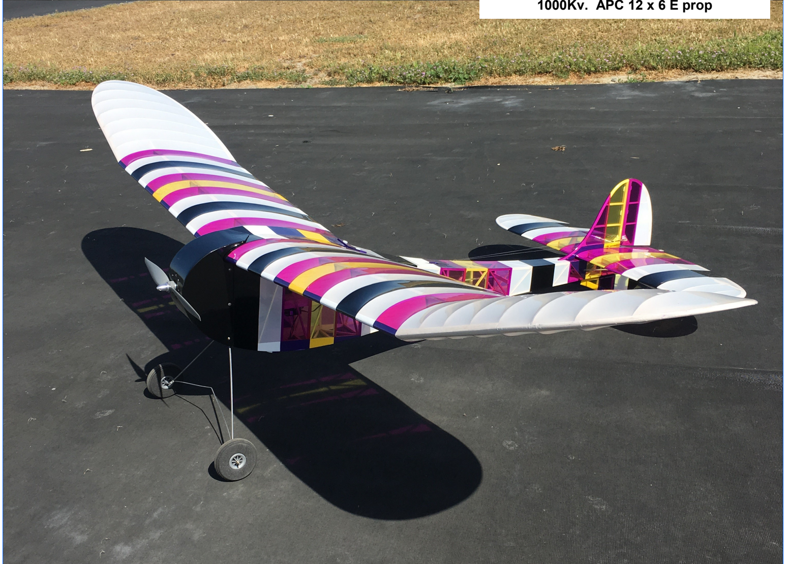
Power: Brushless motor, Suppo BL 2814/8 1000Kv. APC 12 x 6 E prop
