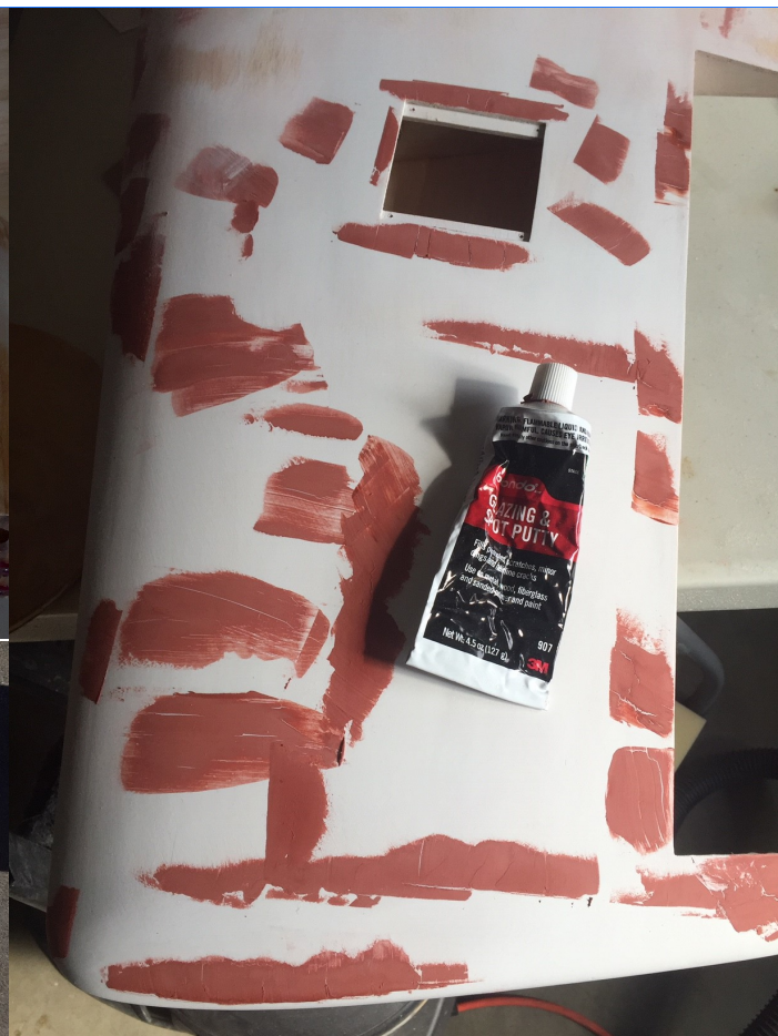
TOP: Top of wing, glassed and sanded. ABOVE: Bottom of wing, freshly primed. RIGHT: Auto spot (glazing) putty applied to every visible low spot, divot, and void. After another sanding and priming, MORE "issues" will be visible!
