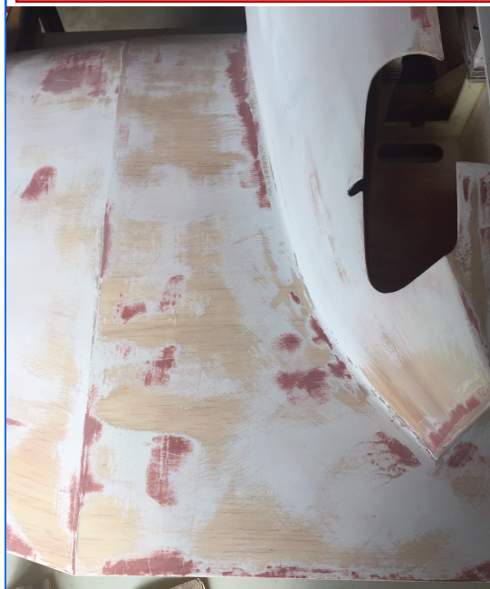
TOP: Top of wing, glassed and sanded. ABOVE: Bottom of wing, freshly primed. RIGHT: Auto spot (glazing) putty applied to every visible low spot, divot, and void. After another sanding and priming, MORE "issues" will be visible!
