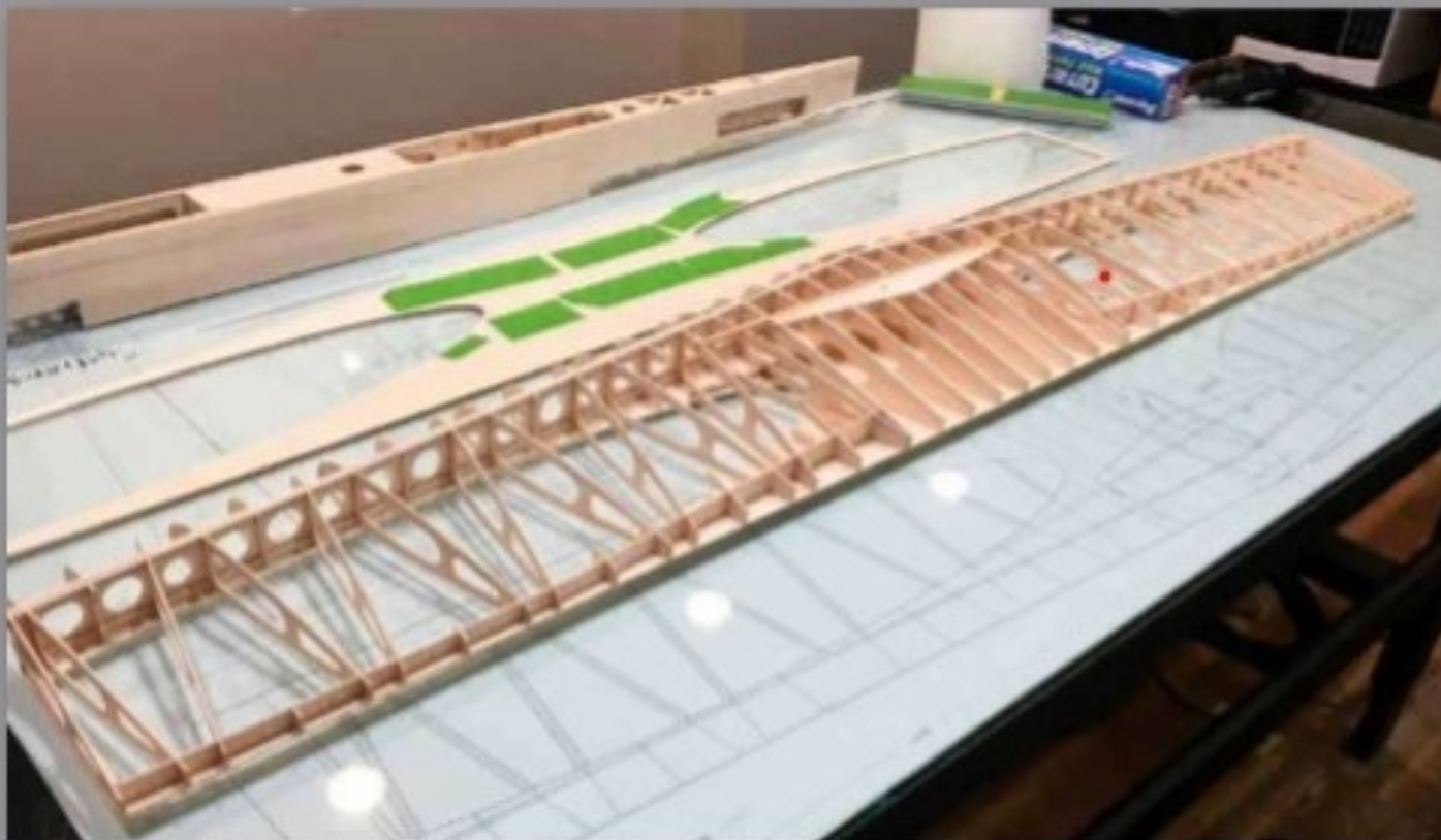
All ribs in place. Full span spar webs with lightening holes and trailing edge webs.
