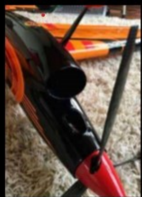
Cooling vent for motor and airscoop which directs air over the ESC.
