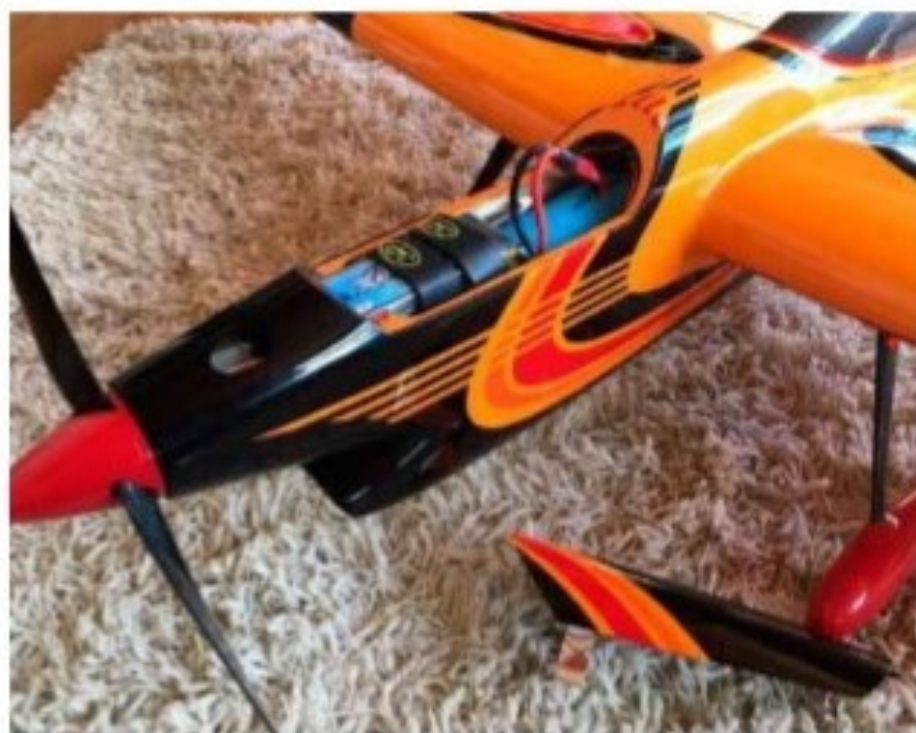
Spring loaded top hatch. "Spring" provided by carbon band in the basic structure.
