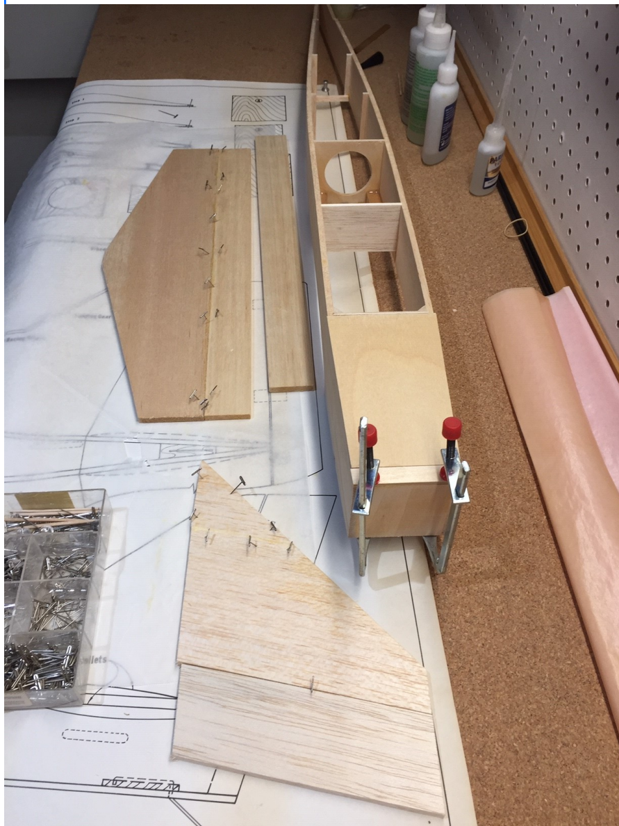
Fuselage and tail parts shown at left.
