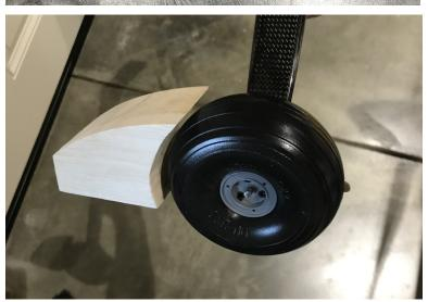
then added blind nuts for mounting the skirts with 6-32 bolts. Additional shaping and sanding ensued until I achieved the desired shape and fit...
