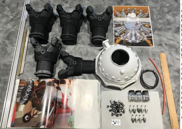
To that end, he employed a 3D printer to create the dummy radial parts, using a quarter scale Williams Brothers R-985 kit as the model. I was shipped the 50% parts and will be painting, 'weathering,' and adding additional scale details to make this dummy come to "life"...
