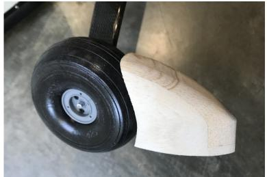
I then added a carbon fiber strip for strength along the length of the skirt and applied fiberglass cloth to all surfaces.
