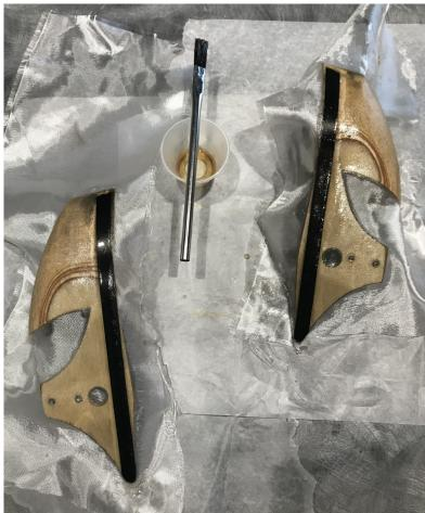
After glassing, it was time to prime, sand, fill, prime, sand, and repeat, until I had a nice smooth paintable finish. Masking, painting, then adding some Goldberg striping tape, I am pleased with the final product, although I have YET to take off or land with these marshmallow tires and low slung skirts... btw: the wheels are DuBro 4.25" Cub wheels. I sanded off and painted over the "Cub" on the hub.
