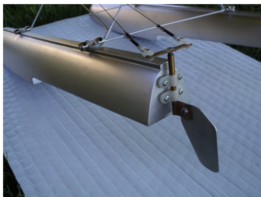
Water-rudder swiveled down in normal operating position before launching.
