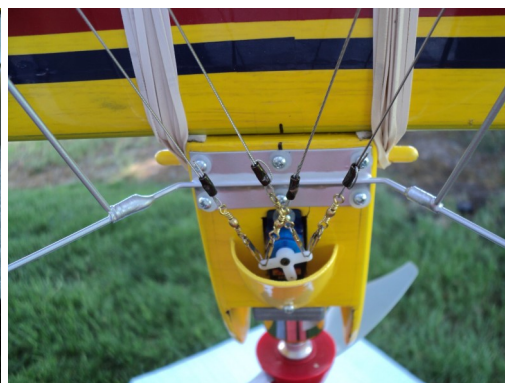
Inexpensive and light-weight fishing tackle used for control system.
