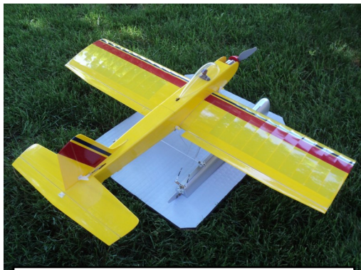
This pad was cut from 3/8" thick foam rubber carpet-pad.
