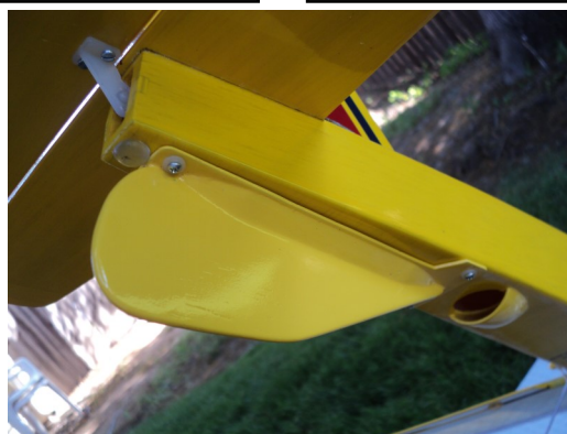
Retracted rudder should clear float- bottom to prevent snagging weeds or driftwood.
