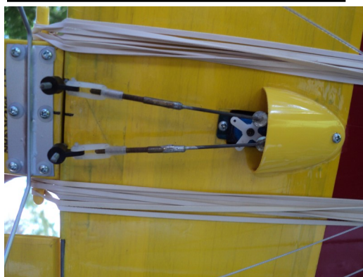
Splash-shield attached with screw (optional) and canopy glue.
