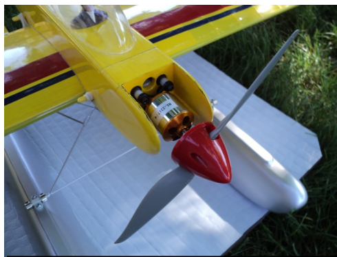
Cheetah A2217-6 Brushless Outrunner Motor (.049 glow engine equivalent)
