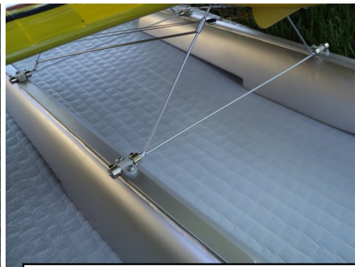
Floats mounted to struts with 5/32" straps and wheel-collars.
