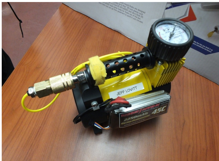
Jeff Lovitt describes the battery-powered compressor he uses to fill aircraft air tanks.
