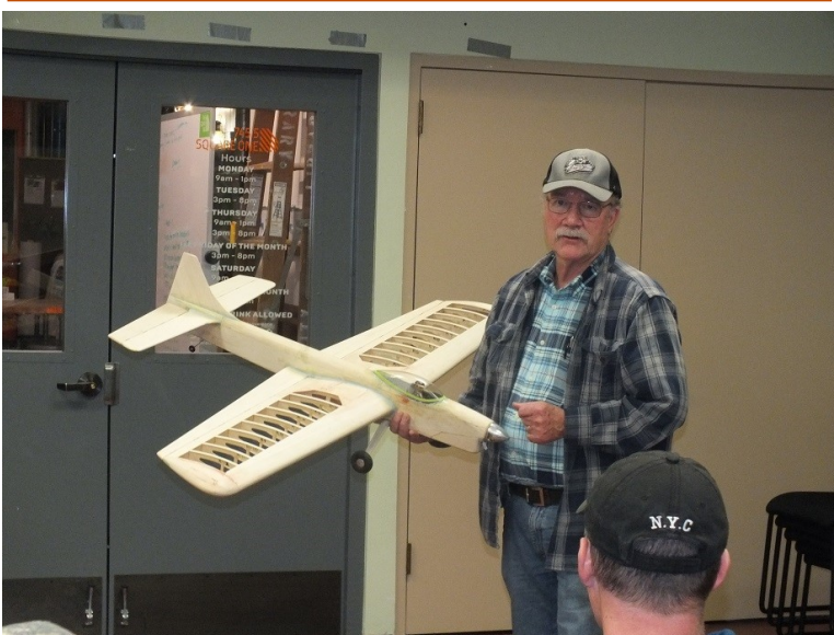
Pete Cunha with a classic control line stunt plane from 1964 called the Skylark. ST .46 ABC with custom muffler and a custom Australian cylinder head. It is covered with carbon fiber veil, Polyspan and butyrate dope and Pete is using Banner wheels that are about forty years old!
