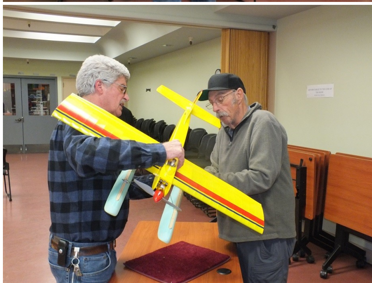
Pete Cunha with a classic control line stunt plane from 1964 called the Skylark. ST .46 ABC with custom muffler and a custom Australian cylinder head. It is covered with carbon fiber veil, Polyspan and butyrate dope and Pete is using Banner wheels that are about forty years old!
