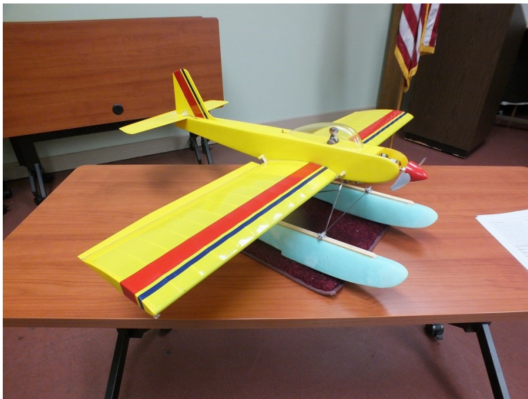
Ed Morgan's SR Batteries XR250 electric sport plane fitted with Hyperion floats. The plane is about the size of a half-A model and was originally designed for a ten cell ni-cad pack. Ed installed a modern out-runner motor and 2S lipo battery. Ed gave several tips on float flying setups and water rudders.
