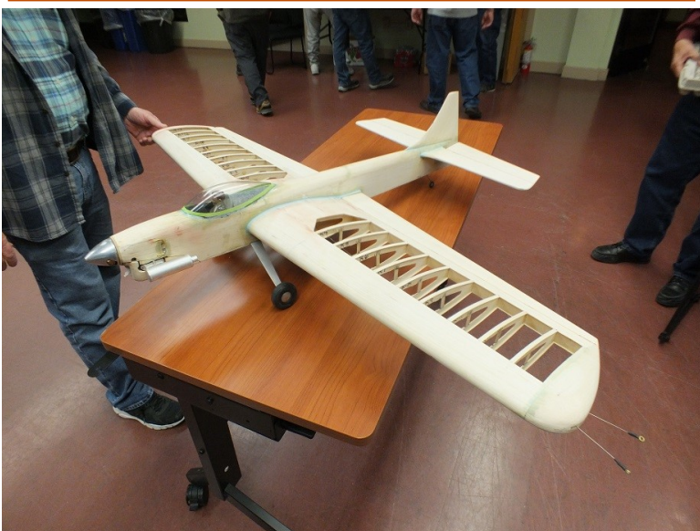
Pete Cunha with a classic control line stunt plane from 1964 called the Skylark. ST .46 ABC with custom muffler and a custom Australian cylinder head. It is covered with carbon fiber veil, Polyspan and butyrate dope and Pete is using Banner wheels that are about forty years old!
