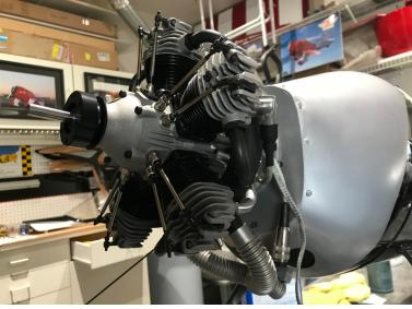
Vogelsang Aeroscale (from whom I purchased the engine) sells a laser cut wood baffle which was positioned, tacked in place, epoxied, filled, then split so as to allow the cowl top and bottom halves to be removed separately. Flexible stainless steel exhaust extensions were added and the cowl opened up for the exhausts at the bottom.
