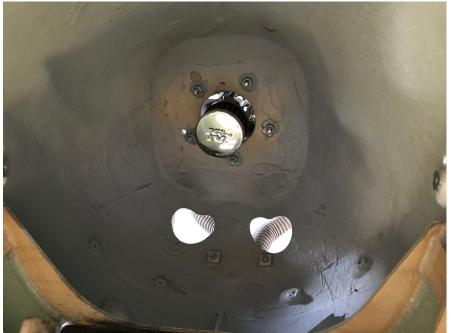
Another very important change to the cowl is the engine baffling. It is critical to limit incoming cooling air so that it MUST pass through the cylinders.
