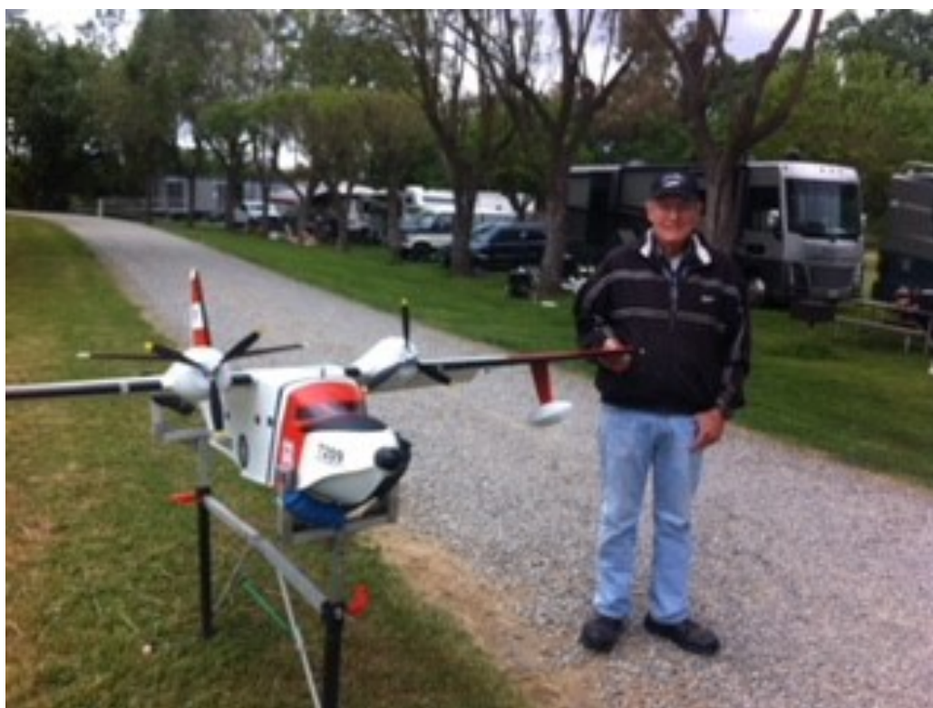
We installed ESC's, motors from my P-38 and props from a Tigercat. Using 2) 4 cell 2600 mAh batteries. Decals from Callie graphics. This is modeled after the Albatross which is currently at the museum at McClellan AF base.
