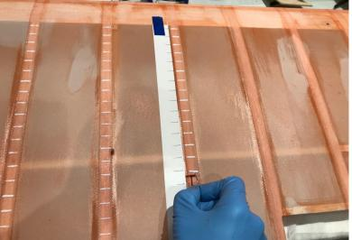
found that adding the look of rib stitching could be easily accomplished using a T-Pin and glue (aliphatic resin or RC 56)
