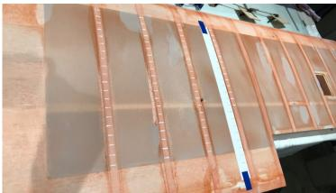
applied on top of the finishing tape. I marked out the scale spacing for rib stitches, which on a third-scale model worked out to a stitch every 17mm. Using the head of the T-Pin, the glue is dabbed directly OVER the pinking tape.
