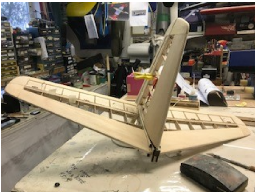
Assembled Horizontal Stab/Vertical Fin and elevators.
