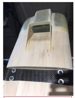
Scale cool air exit vent on the underside of the cowl/fuselage
