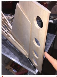
I embedded a carbon fiber rod in the balsa rudder trailing edge primarily to protect it from hangar rash, secondarily to stiffen the rudder.
