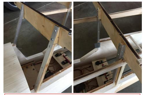
Aluminum angle stock glued and screwed to the hardwood cabin uprights—which support the wing... then through-bolted to the ply wing center sections.
