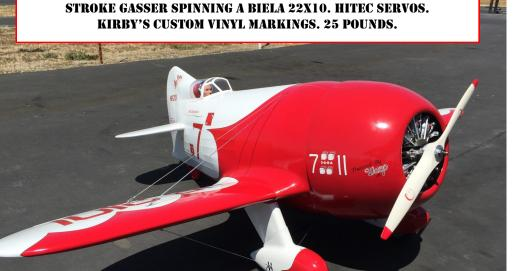
BYRON GEE BEE R2: FIBERGLASS FUSELAGE, BUILT-UP AND GLASSED WINGS (SCALE 75" SPAN). NEAR SCALE STAB SPAN. SAITO 61CC 4
