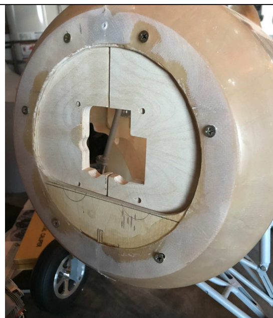
After cutting firewall into two pieces and installing behind fuselage nose ring
