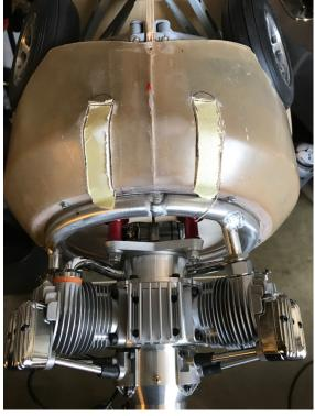
Once the reliefs were created, I then found that fairly large portions of wood also needed to be removed from the firewall halves to create the clearance required for the exhaust stacks. Thanks goodness for Dremels and carbide sanding drums!
