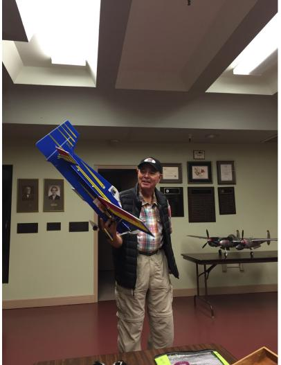
Lou Fox showed off his Laser 200 "flatty" from Tower Hobbies. With a 33.5" span and made from 3mm depron foam, Lou said the model is very fragile. The Laser features generous use of carbon fiber reinforcement struts. The 250 size brushless motor and 12A ESC were acquired from Hobby King. Ready to fly weight is about 6 ounces.
