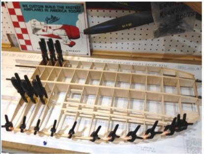
As for the building of the Byron, the kit is a bit of a departure, as the wing halves are totally built-up from laser cut ribs, typical top and bottom spruce and balsa spars plus full length sheer webs, all assembled on fiberglass arrow-shafts. The wing also incorporates some wash-out. Being a bit "rusty" on the building board, I have found myself making some dumb mistakes... nothing critical, but indicative of being away from read-
