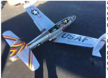
age to the nose inlet area... all easily repairable. The wing, however, is another matter. The rear strut attachment glue joints failed inside the wing, and when those failed it bent the forward spar at the angle you see in the picture.
