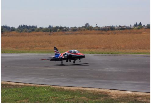
about 3 seconds! I was unable to fly the plane due to severe yaw oscillations, and was unable to switch off the iGyro because I didn't have a mental plan for what I would do if things were not right. The result was a loss of airframe and major damage to the engine. Pride severely bruised. I've had some time to think about what happened now. The root cause was a rush to fly. I was mov-
