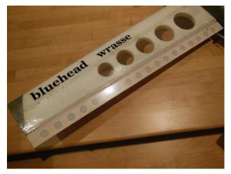
The wing comes shaped but needs to be sanded and stiffened with carbon rods top and bottom. It is covered with a material called "new stuff".
