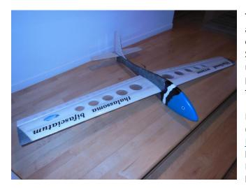
This model called the "le Fish" is an EPP foam slope unlimited aerobatic glider. It has a 66 inch wing span and weighs 30 ounces. The air foils are a blend of airfoils- SB96V (root) and SB96VS (tip) for better inverted performance and versatile allround capability. The wing loading is 10-11 oz. per sq. ft. My plane has been extensively lightened with lightening holes on the control surfaces and wing.
